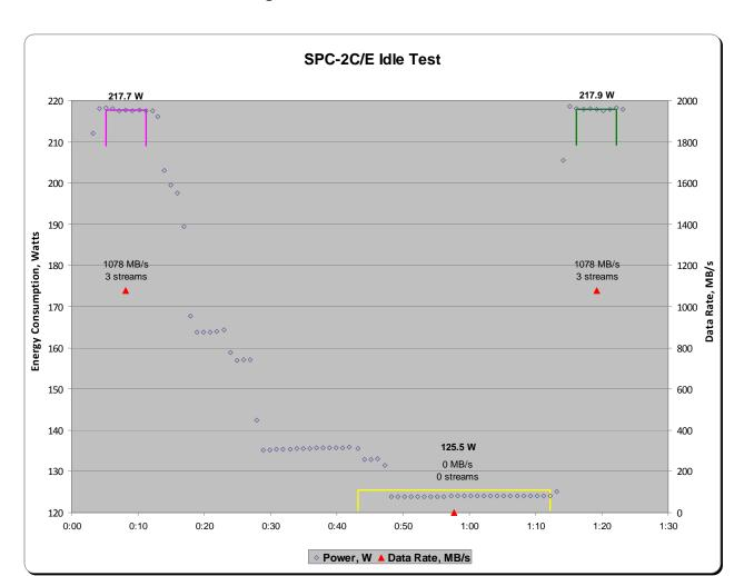
Figure 12-1: SPC-2C/E Idle Test
