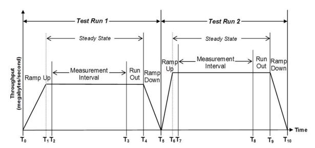
Figure 6-1: SPC-2C Test Run Components
