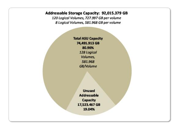
Figure 10-14: SPC-2C Total Unused Storage Capacity Ratio and Detail
