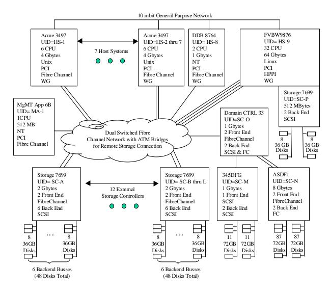
Figure 10-10: Benchmark Configuration/Tested Storage Configuration Diagram
