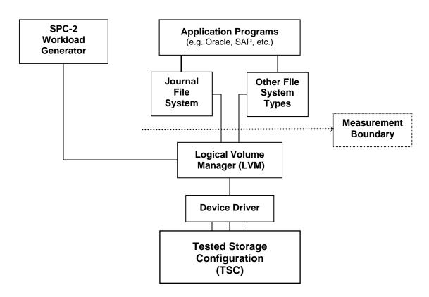
Figure 5-2: Measurement Boundary in an UNIX System Implementation
