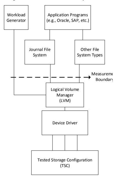
Figure 5-4 Measurement Boundary
