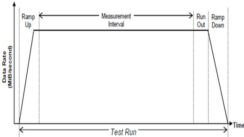
The IO load presented to the TSC during a TEST PHASE may be zero and a TRANSITION may occur either from or to an I/O load of zero. The load levels shown during the transition portion of the figure are for illustration only and reflect a typical case.
