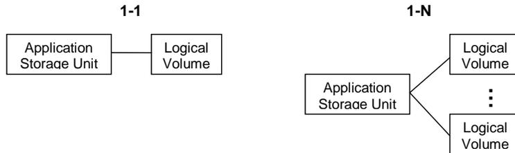
**Figure 2-1: ASU-to-Logical Volume Address Mappings**
