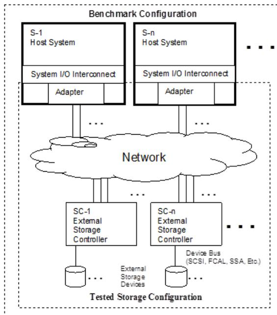
4.4.6 **Network Storage – External Storage Controller and External Storage Devices**
